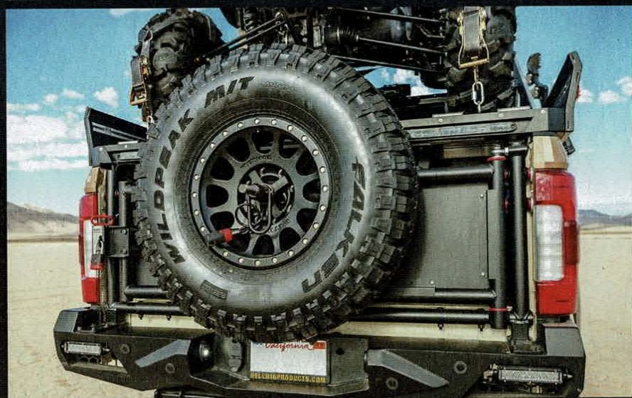
▲ Replacing the factory tailgate is a unit from Wilco Off-Road which houses the spare, a 37-inch tall Falken meat mounted on Method wheel.
