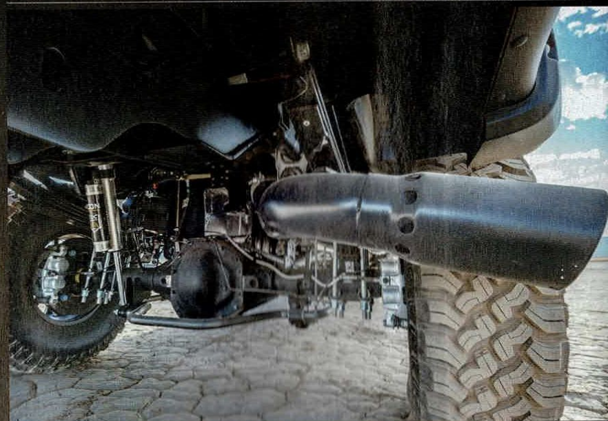
▲ Out back, Icon got the nod as well for suspension duties. Here again resides an upgraded Hellwig swaybar for improved handling. A Magnaflow DPF back exhaust system is used to help the 0.7L breathe a bit easier.
