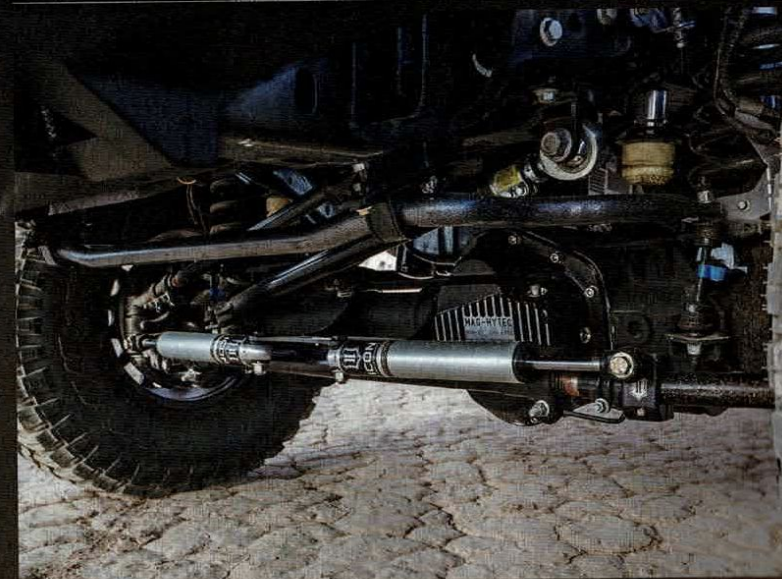
▲▲ A suspension system from Icon keeps the F350 capable in the dirt while a Hellwig swaybar keeps the heavy load level in the turns. Mag-Hytec differential covers help protect the differentials both inside and out.
